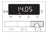
The Duration → and End → function indicators light up and the temperature is shown in the display.
